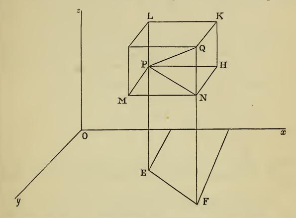
parallel to each of the co-ordinate planes, thus forming a parallelepiped whose edges are parallel to the co-ordinate axes, and are equal in length to  $x_2 - x_1$ ,  $y_2 - y_1$ ,  $z_2 - z_1$ , respectively.
